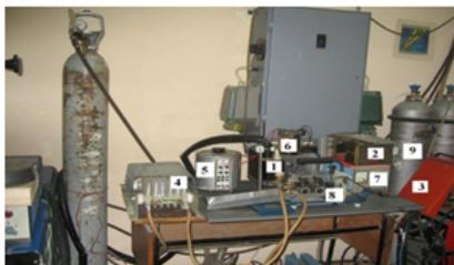
Fig. 3. Experimental setup used for production of iron microparticles in plasma. 1 - plasma generator (intensity of electric current is max 600 A<sub>c</sub>), 2 - rectifier bridge, 3 - power source (max 110 A<sub>c</sub>), 4 - power resistance (2Ω/3kW), 5 - autotransformer, 6 - separator transformer, 7 - power supply, 8 - advance system, 9 - argon storage under pressure (130 bar).
