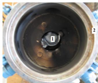
Fig. 6. Plasma generator after spraying the iron rod. 1 - Iron rod, 2 - Plasma generator block.
